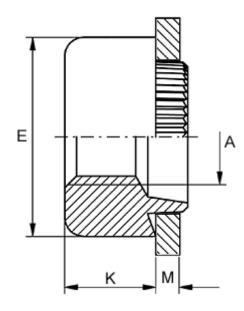
Female thread A = M14Height K = 10.0Outer diameter E = 25.0Plate thickness = 2.0 to 2.2
